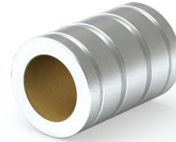
Along with not absorbing water and being affected by swelling, the bearing liner materials are **self-lubricating** and eliminate the need for external lubrication. Not requiring lubricants, even food grade type grease and oil, decreases the amount of material deposits and buildup on the shaft surface, and the potential for bacteria buildup.
